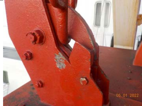
Stbd side L/B forward part link stopper stuck due to paint.
