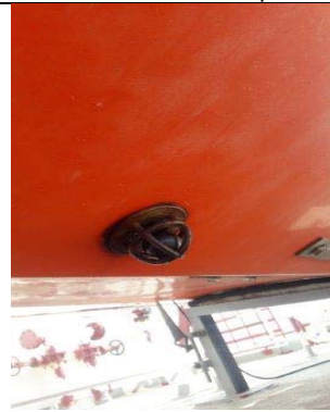
Stbd side L/B forward part link stopper stuck due to paint.
